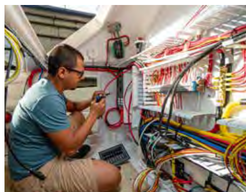
FINISH ELECTRICAL Christian Osorio wires the helm inside the console of a 72 Convertible.
