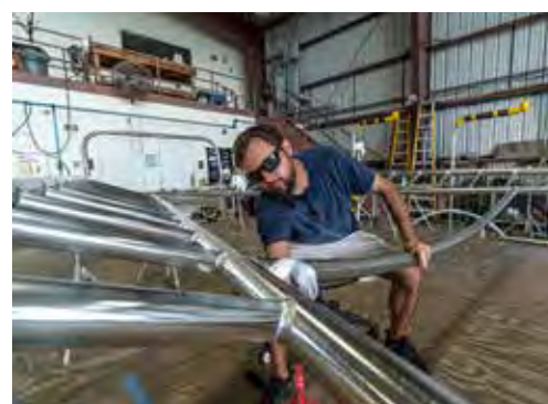
Curtis Updike cleans up the hardtop aft perimeter rail before welding the rail to the tower inner leg.
